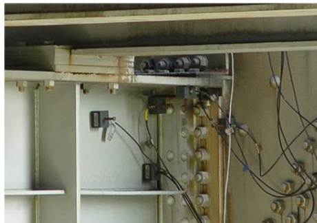
Fig. 3. Data and Guard Sensors on I-10 Mississippi River Bridge (Baton Rouge, LA)
