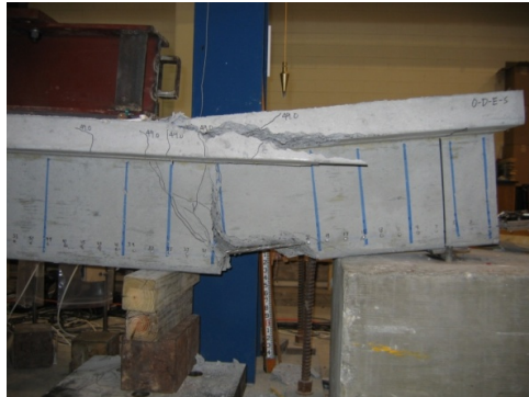
Fig. 10. Shear-Tensile Failure in Prestressed Girder Specimen (after Xu, 2008)
