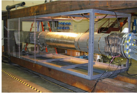
Fig. 7. Suspension Bridge Cable Test Cell with Multiple Sensor Types
